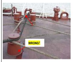
The effectiveness and safety of the moorings is dependent upon the configuration of the mooring lines. Officer in charge should be familiar with configuration of the moorings, so *that leads are effective and do not create sharp angles*.
