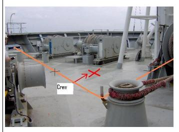
The orange line shows the wrong arrangement of the rope while heaving up. It should never be attempted to heave up the rope this way!!! The rope must always work against the roller and roller must move freely (well greased).
