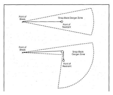
Always keep on mind that rope can break and snapback, especially synthetic rope, when under the load/stress. Treat every synthetic rope under load with extreme caution! Synthetic ropes normally break suddenly, without warning, without audible signs. Stand clear of potential path of snapback whenever possible. The potential
