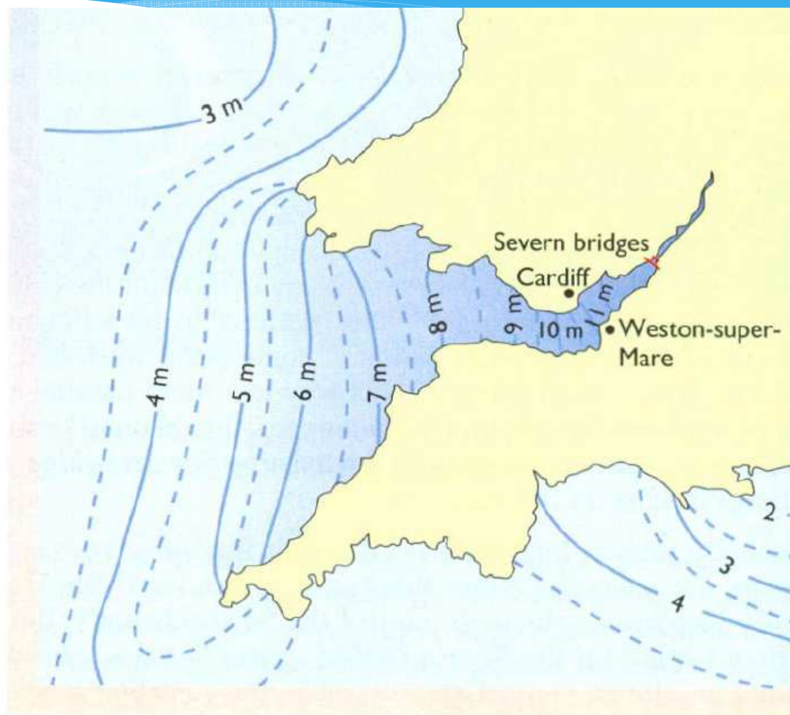
Figure 6.5 The effects of concentration of tidal flow in the Severn Estuary (tidal ranges in metres)
