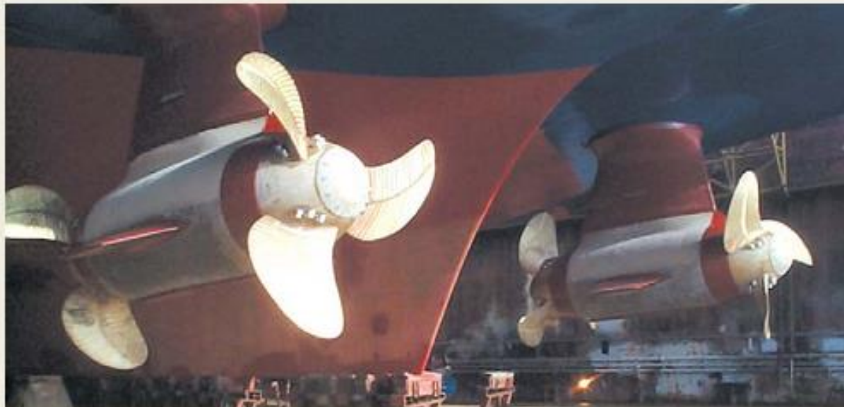
Siemens-Schottel SSP propulsion system
