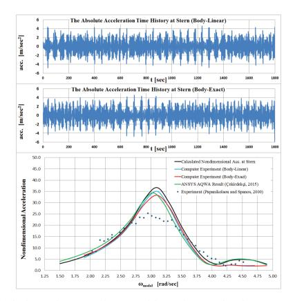
Fig. 13 The absolute acceleration time histories and the non-dimensional acceleration at stern (ITTC-2)
