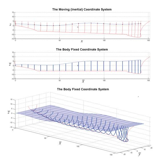
Fig. 1 Body-exact strip theory calculation
