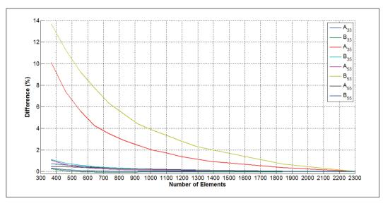
Fig. 2 Convergence test sample (Encounter Wave Frequency = 1.1106 rad/sec)
