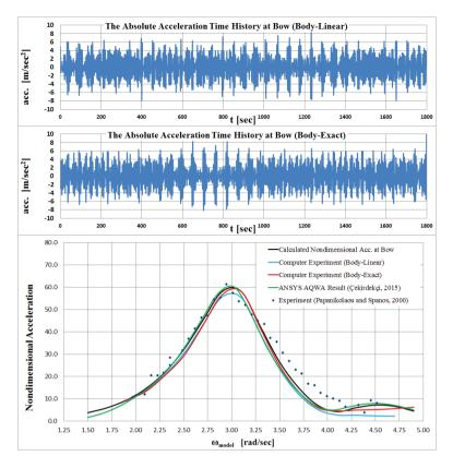
Fig. 12 The absolute acceleration time histories and the non-dimensional acceleration at bow (ITTC-2) Source: Authors
