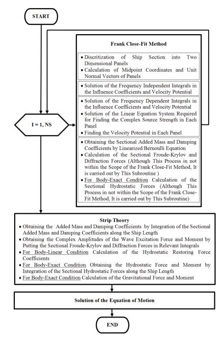
Fig. 4 Flow diagram (calculation of the RAO ordinates subroutine)
