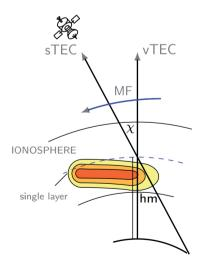
Figure 2 Thin shell approximation of the ionosphere
