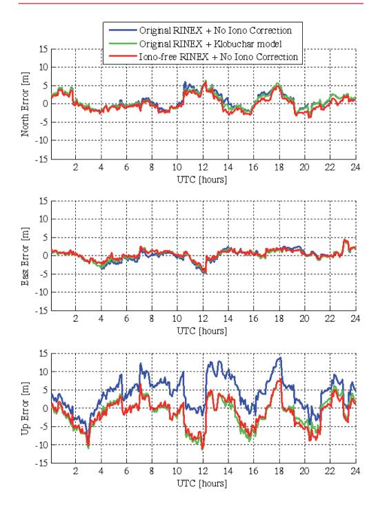
Figure 2 Positioning error in north, east and up direction for different positioning methods on ZGRB station, 10 August 2014
