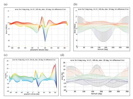
**Figure 4** Mapping function error depending on geographical latitude (a) and azimuth (b) in absolute values and in percentage (c, d)
