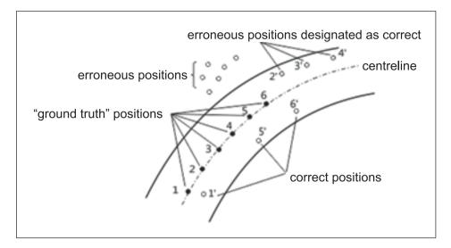
Figure 5 Accuracy measurement methodology
