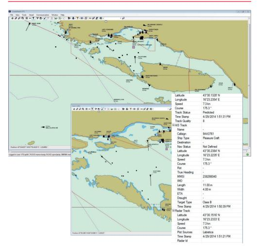
Figure 9 An example of AIS Class B target – leisure craft displayed on Electronic Navigational Chart (ENC) (SAAB CoastWatch VTS Software)
