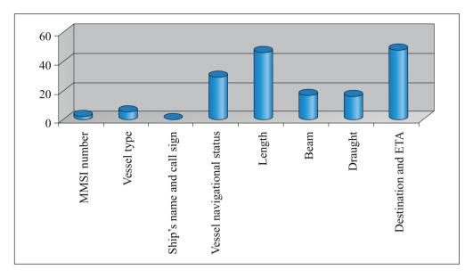
Figure 5 The most common AIS message errors, given in percentage
