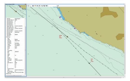
Figure 3 Presentation of AIS Class B on the VTS operator's control display (SAAB CoastWatch VTS Software)
