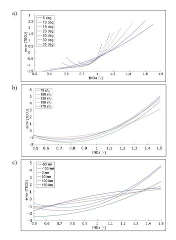
Figure 8 Variation of mapping function error depending on asymmetry index for changing solar radio flux (a), elevation angle (b) and ionospheric height (c)
