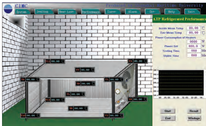
Fig. 9. ATP refrigerated performance test
