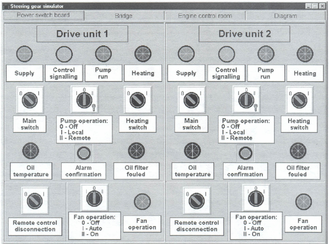
Fig. 6 Steering gear simulator – Power switch panel
