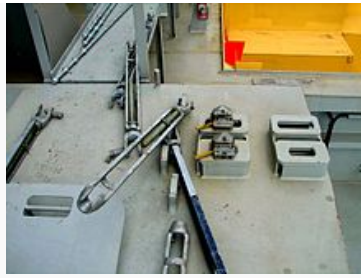
Twist-locks and lashing rods ( pictured ) are widely used to secure containers aboard ships.
