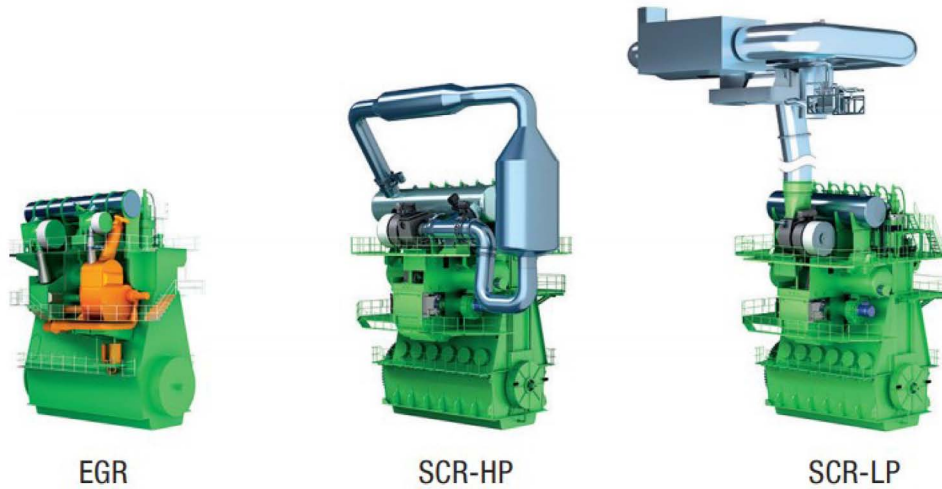
Figure 4 EGR and SCR HP and LP dimensional differences [3]
