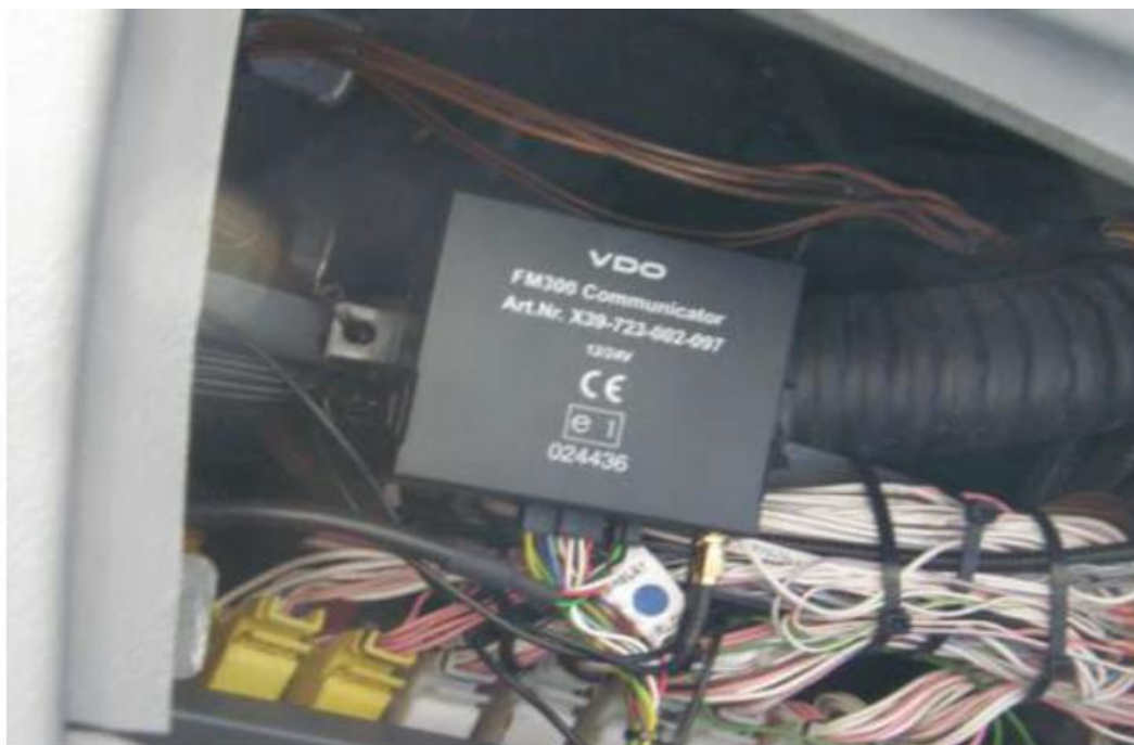
Slika 26. Simens VDO Fleet Manager 300 Communicator
